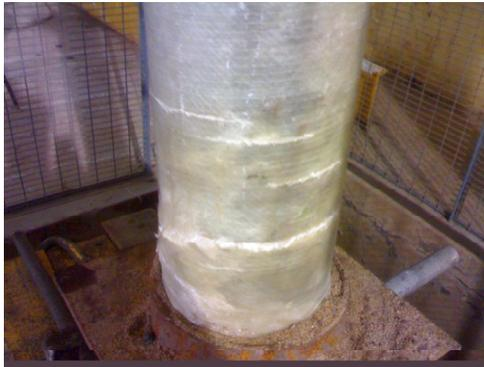
Fig. 6. Failure status of UDC
