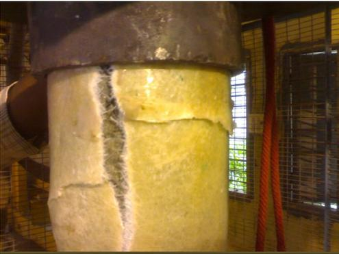
Fig 5. Failure status of CSM
