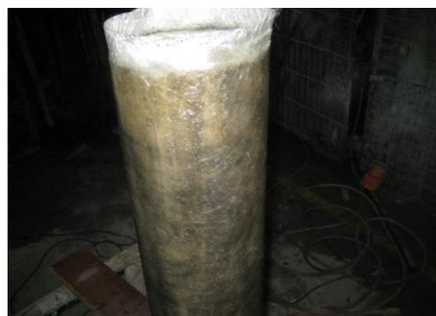
**Fig. 3. GFRP Wrapped Specimen**
