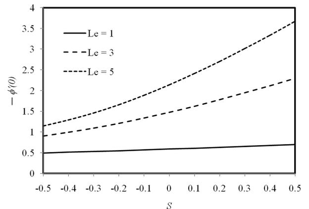
Fig. 27. Variation of  $\phi'(0)$  with  $S$  for different  $Le$
