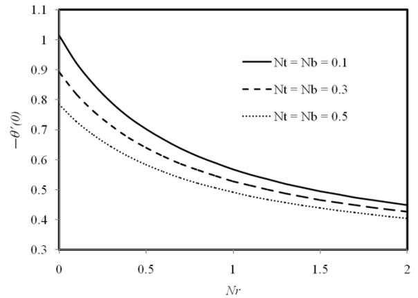
Fig. 26. Heat transfer versus  $Nr$  for different  $Nt$  and  $Nb$
