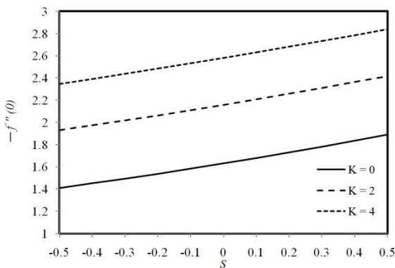
Fig. 23. Skin friction versus  $S$  for different  $K$
