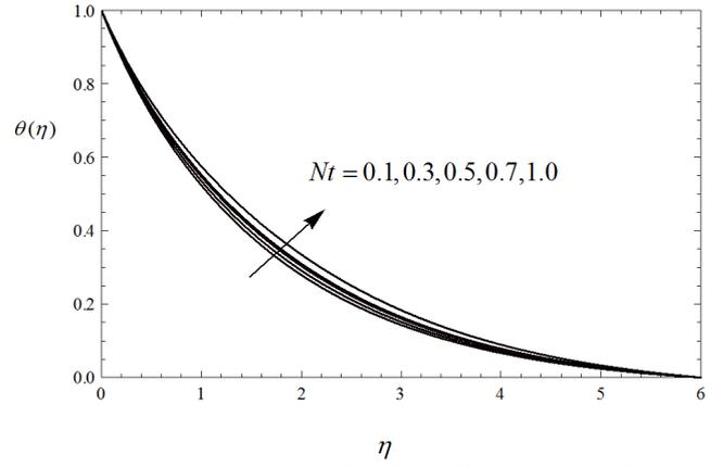
Fig. 16. Temperature profiles for different values of Nt
