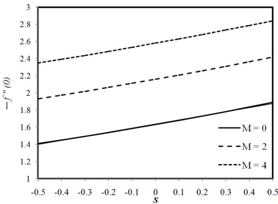
Fig. 22. Skin friction versus  $S$  for different  $M$
