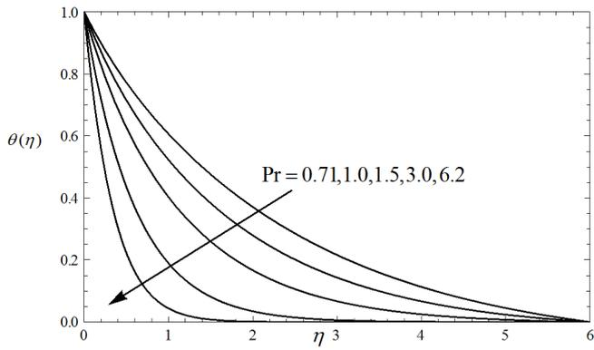
Fig. 12. Temperature profiles for different values of Pr
