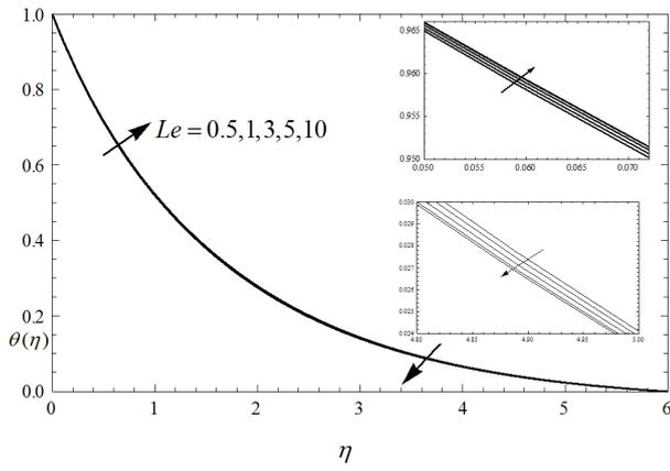
Fig. 20. Temperature profiles for different values of  $Le$
