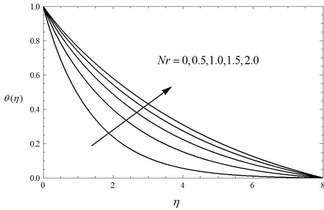
Fig. 14. Temperature profiles for different values of Nr
