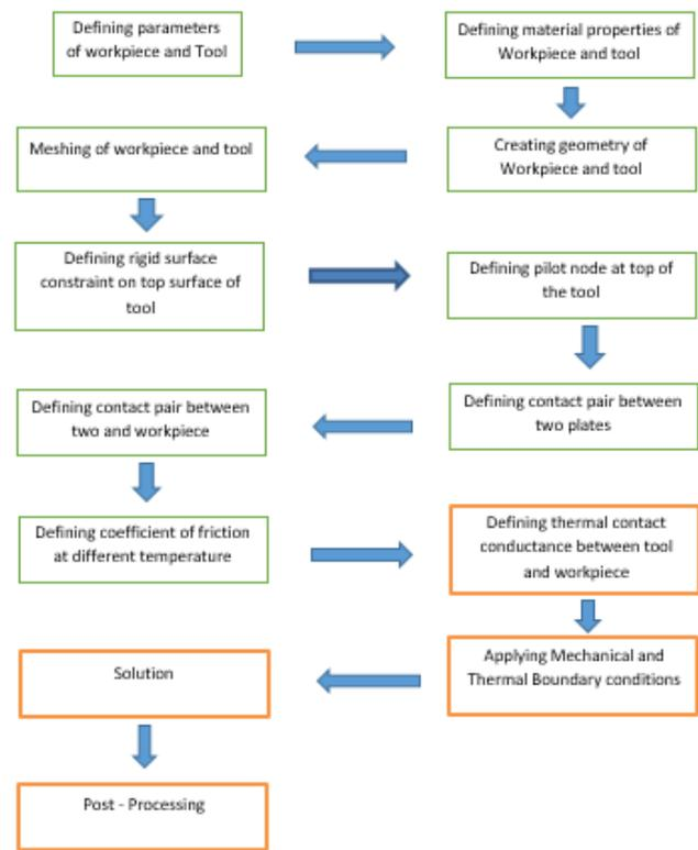
Fig. 1. Layout for model creation and performing analysis using Ansys
