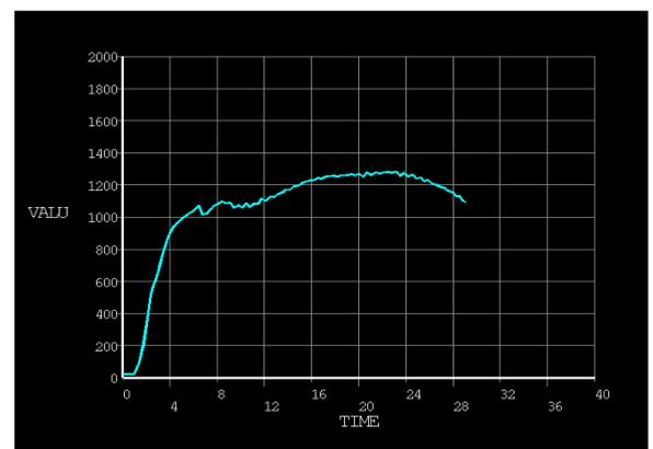
Graph 4.4 Frictional heat vs. Time (66 rpm)
