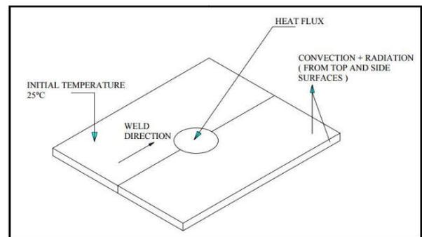
**Fig. 3. Schematic representation of boundary condition for thermal analysis**
