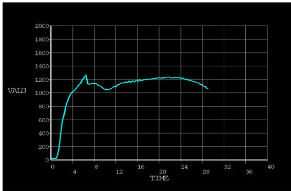
Graph 4.6 Frictional heat vs. Time (78 rpm)
