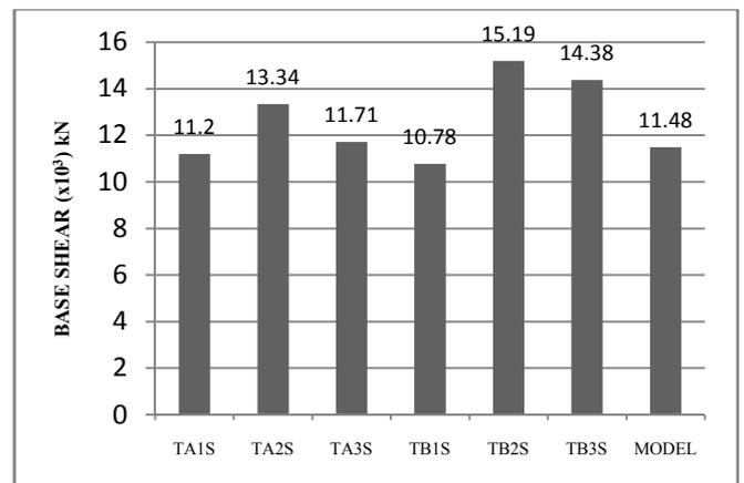
**Fig. 5. Maximum Base shear with steel bracings**
