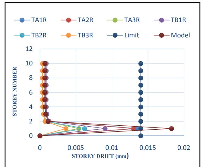
Fig. 9. Storey drift with RCC bracing
