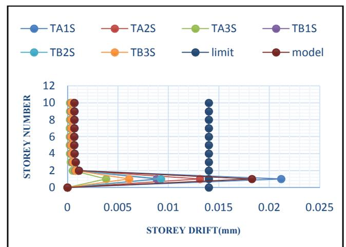
Fig.10. Storey drift with steel bracing
