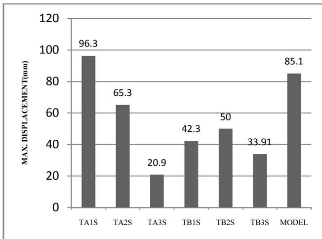
Fig. 7. Maximum displacement with steel bracing
