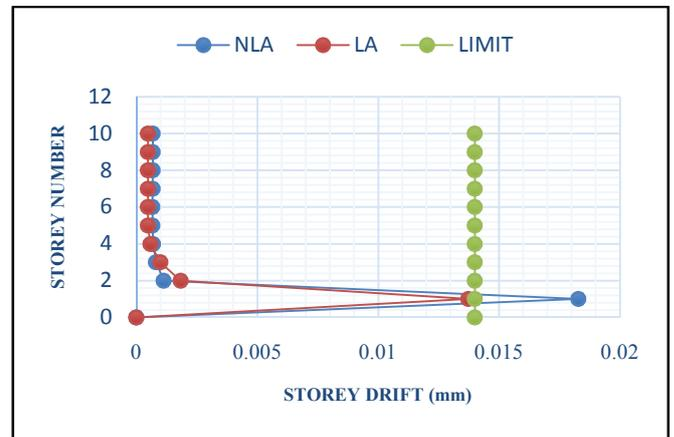
Fig. 8. Storey drift with linear and non-linear analysis
