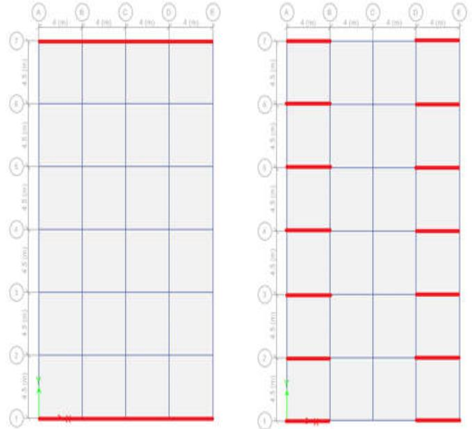
**Fig. 3. Plan of Type A and Type B model**
