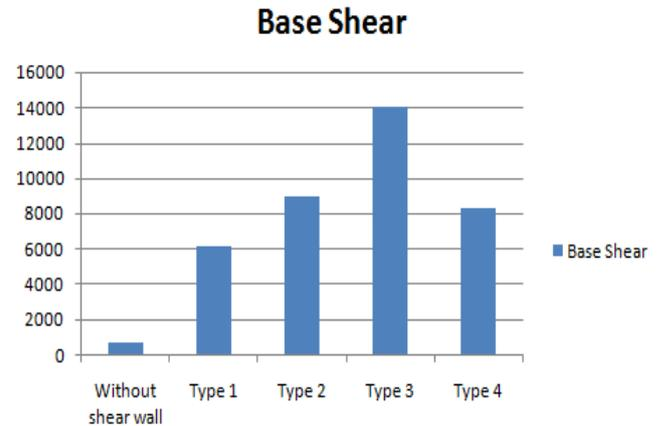
Fig. 8. Maximum Base shear
