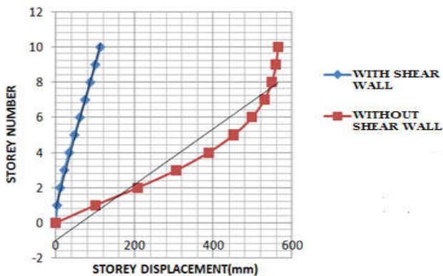
Fig. 7. Storey displacement of building with and without shear wall by using push over analysis
