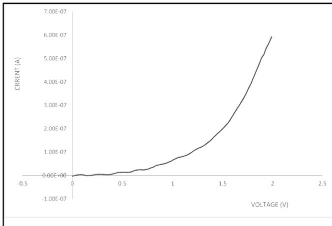
Fig. 2. I-V Characteristics of ITO/ZnS/SnS/Ag Solar cell (in the dark)
