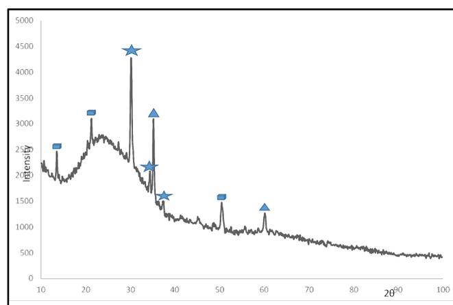
Fig. 1. XRD Pattern of ZnS/SnS heterojunction on ITO coated glass (SnS ZnS ITO)
