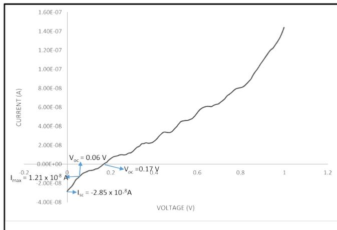
Fig. 3. I-V Characteristics of ITO/ZnS/SnS/Ag solar cell (under illumination)
