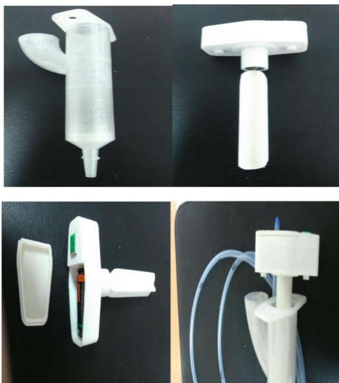
Figures 3 . Model of NG feeding equipment for electronic stirring
