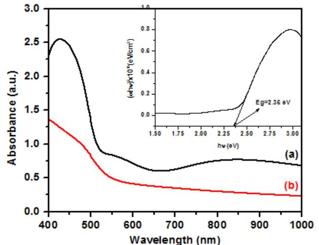
Fig. 3. Room temperature optical absorption spectra of nanocrystalline CdS thin films prepared by using CBD and SILAR technique
