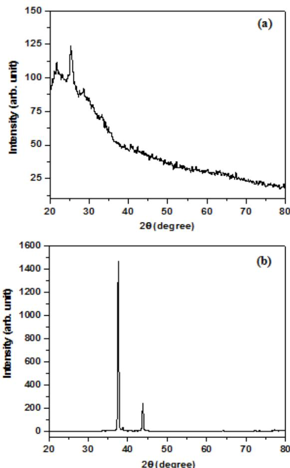
Fig. 1. XRD Patterns of nanocrystalline CdS thin films prepared by using (a) CBD and (b) SILAR technique
