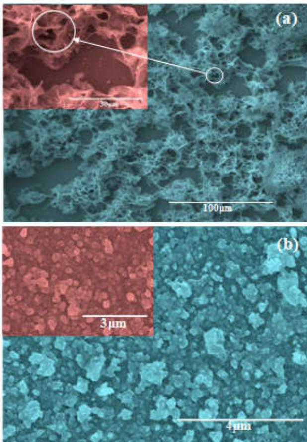
Fig. 2. FE-SEM images of nanocrystalline CdS thin films prepared by using (a) CBD and (b) SILAR technique
