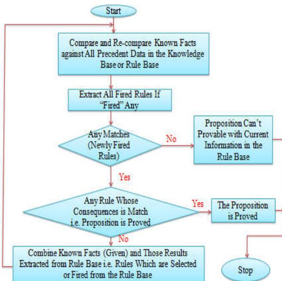
Fig. 3. Flowchart of Forward Reasoning Process
