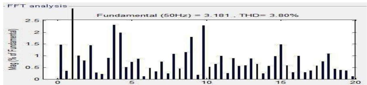
Fig. 17. Current harmonics for without transformer connection
