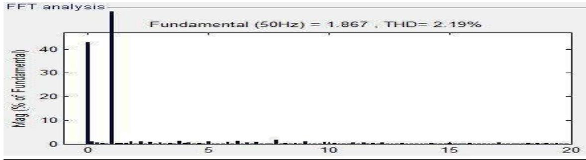
Fig 7. Current harmonics after transformer for Connection A
