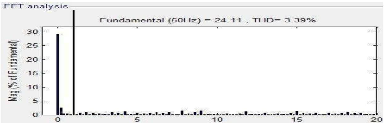
Fig 13: Current harmonics after transformer for Connection B
