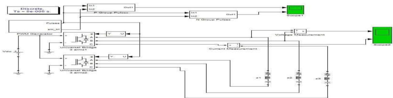
Fig. 15. Simulink model without transformer connectio
