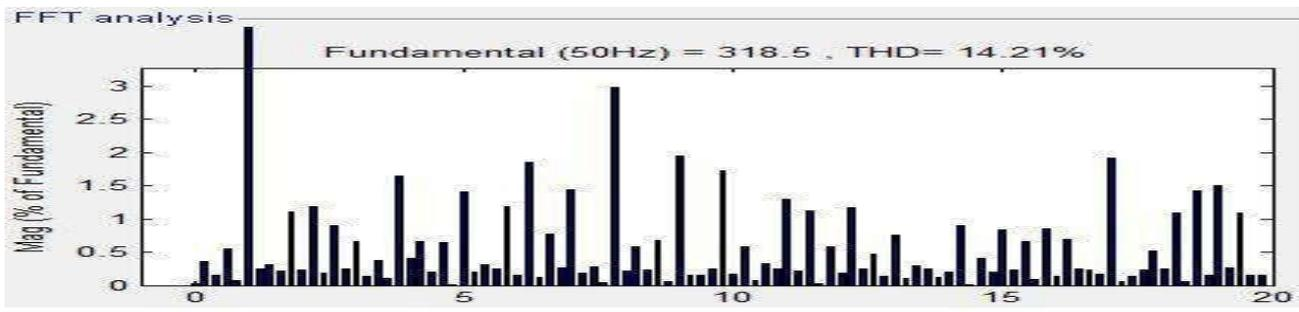
Fig 4. Voltage harmonics before transformer for Connection A
