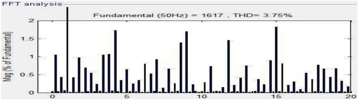
Fig 12: Voltage harmonics after transformer for Connection B
