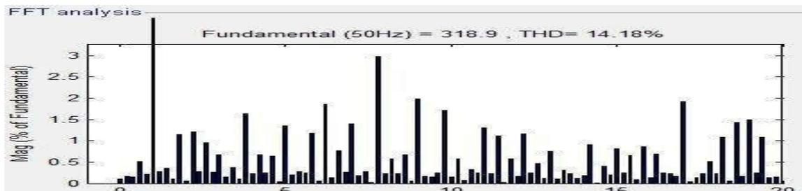
Fig 10: Voltage harmonics before transformer for Connection B
