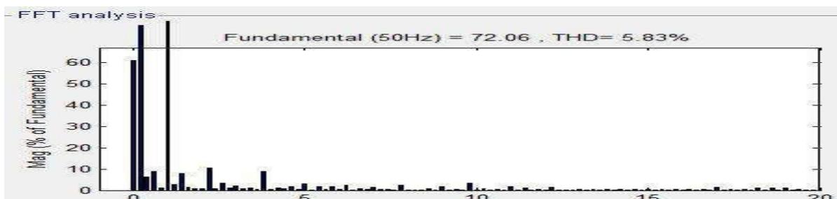
Fig. 11. Current harmonics before transformer for Connection B
