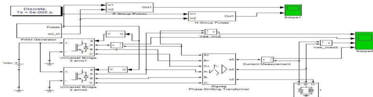
Fig 9: Simulink model of Connection type B
