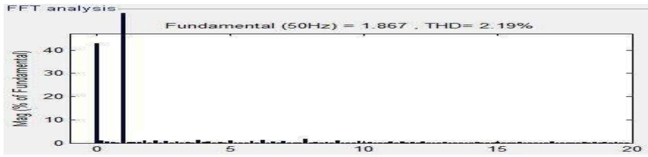
Fig 5. Current harmonics before transformer for Connection A
