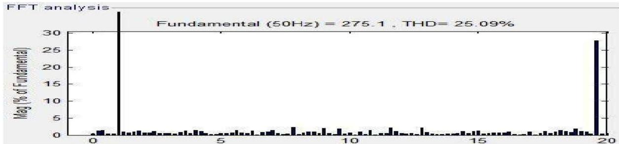
Fig. 16. Voltage harmonics for without transformer connection
