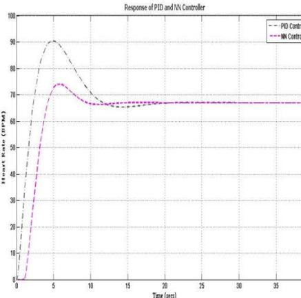
Figure 4. Response of PID and NN controller for 67 and 72 bpm
