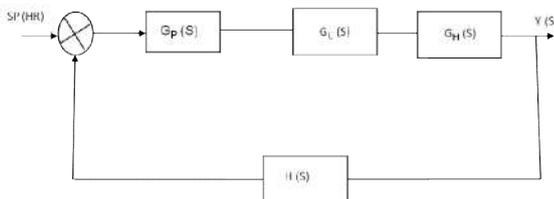
Figure 5. Block diagram of Cardiovasular Control Scheme
