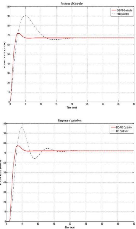
Figure 6. Response of PID and Bioinspired tuned controller
