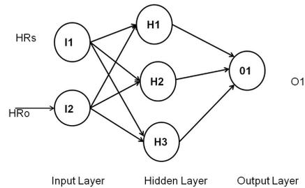
Figure 3. Architecture of Proposed BP NN control scheme
