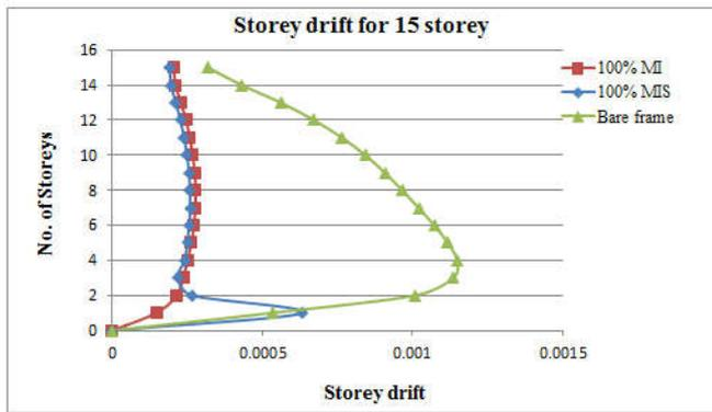
Fig. 12. Storey drift of 15 storey building for fully infilled frame, soft storey and bare frame models in zone V
