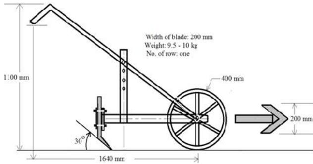
Figure a. Wheel hoe with sweep type blade
