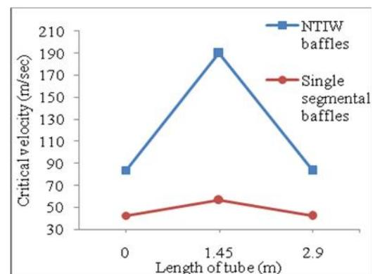
Figure 3. Critical velocity vs length of tube
