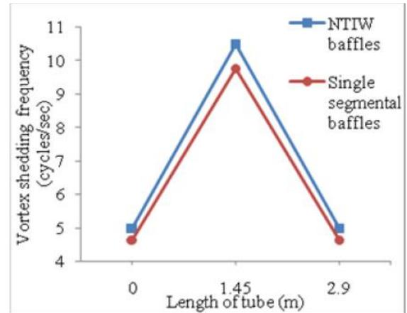
**Figure 5. Vortex shedding frequency vs length of tube**
