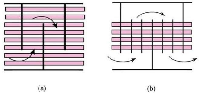
Figure 1. Types of baffles used: (a) Single segmental baffles and (b) Single segmental baffles with no tubes in windows
