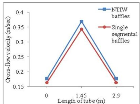
Figure 2. Cross-flow velocity vs length of tube
