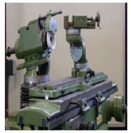
Fig. 16. Tool and cutter grinder
