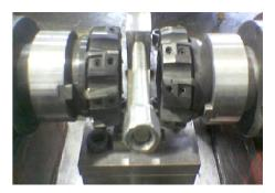
Fig. 8. Duplex milling machine
