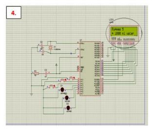
Fig.9. In this the LCD will display the amount and respective quantity of water. For Rs.5 it will give 1000ml water
