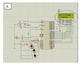
Fig.10. In this the LCD will display the message after the coin of Rs. 1 is inserted. Here encircled switch is considered as input for Rs.1.
