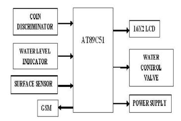
Fig.2. Block Representation of proposed system
