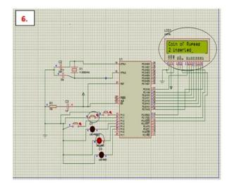
Fig.11-In this the LCD will display the message after the coin of Rs. 2 is inserted. Here encircled switch is considered as input for Rs.2.
