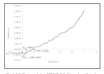
Fig. 3. I-V Characteristics of ITO/ZnS/SnS/Ag solar cell (under illumination)
