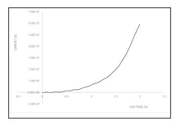
Fig. 2. I-V Characteristics of ITO/ZnS/SnS/Ag Solar cell (in the dark)
