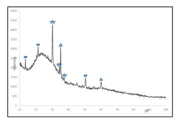
Fig. 1. XRD Pattern of ZnS/SnS heterojunction on ITO coated glass (SnS ZnS ITO)
