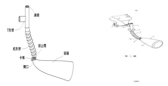
Figure 13. Design of the assisting components of sputum drainage of the trachea
