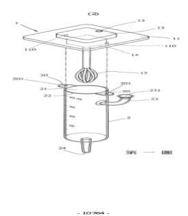
Figure 2. Design of NG feeding equipment for electronic stirring
