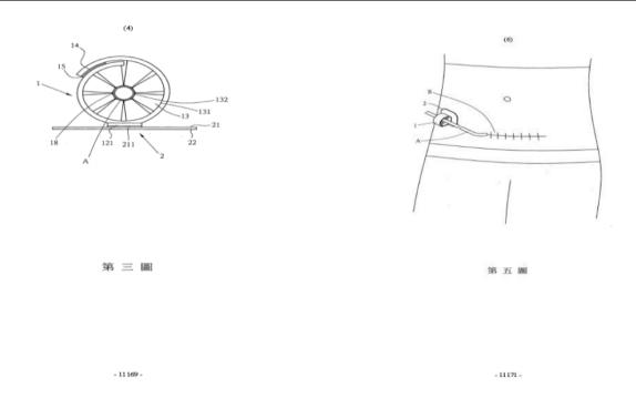
Figure 9. Design of the tube fixation device
