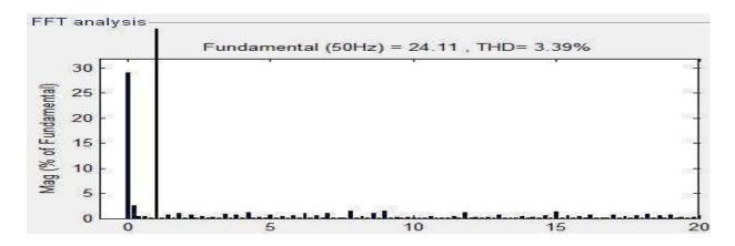
Fig 13: Current harmonics after transformer for Connection B
