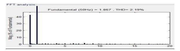
Fig 7. Current harmonics after transformer for Connection A
