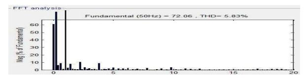
Fig. 11. Current harmonics before transformer for Connection B
