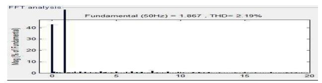
Fig 5. Current harmonics before transformer for Connection A
