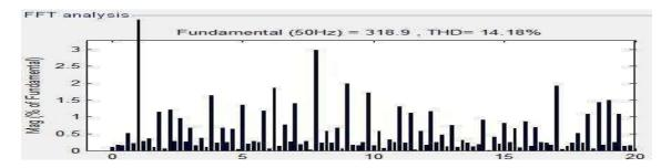
Fig 10: Voltage harmonics before transformer for Connection B
