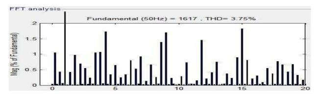
Fig 12: Voltage harmonics after transformer for Connection B
