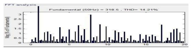
Fig 4. Voltage harmonics before transformer for Connection A
