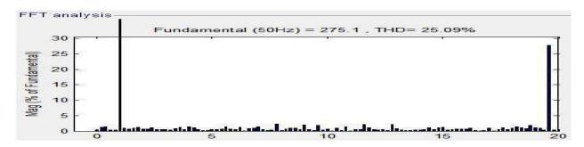
Fig. 16. Voltage harmonics for without transformer connection
