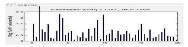
Fig. 17. Current harmonics for without transformer connection
