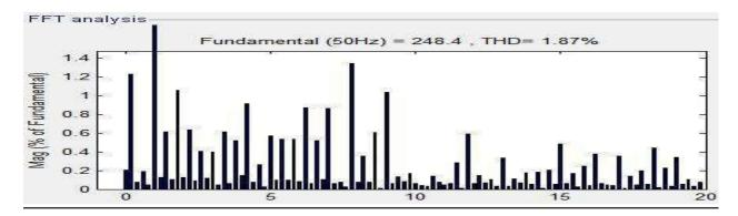
Fig 6. Voltage harmonics after transformer for Connection A
