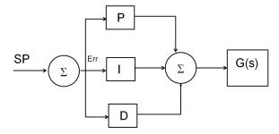
Figure 1. Feedback PID Controller
