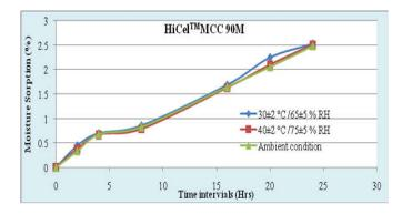
Fig. 5. Moisture sorption in percentage of HiCel<sup>TM</sup>MCC (Microcrystalline Cellulose)
