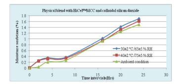
Fig. 7. Moisture sorption in percentage of Physical blend with HiCel<sup>TM</sup>MCC and colloidal silicon dioxide
