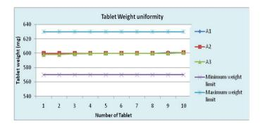
Fig. 1. Weight uniformity of Acetyl salicylic acid tablet (A1- tablet manufacturing with HiCel<sup>™</sup>MCC, A2- HiCel<sup>™</sup>SMCC and A3- Physical blend)
