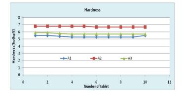
Fig. 2. Hardness of individual Acetyl salicylic acid tablet (A1tablet manufacturing with HiCel<sup>™</sup>MCC, A2- HiCel<sup>™</sup>SMCC and A3- Physical blend)
