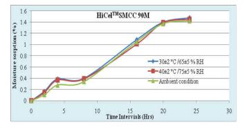
Fig. 6. Moisture sorption in percentage of HiCel<sup>TM</sup>SMCC (Silicified Microcrystalline Cellulose)
