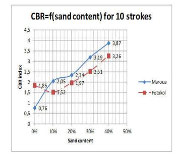
Figure 7. CBR index according to sand content for 10 strokes (K1 or K2)
