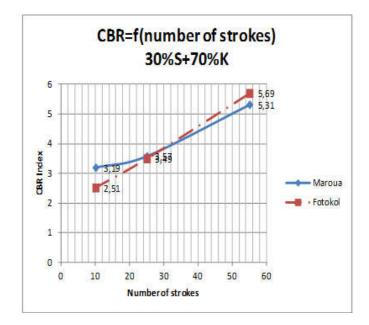
Figure 5. CBR Indexes according to the number of strokes for compounds 20%S+100% (K1 and K2), 30%S+90%(K1 and K2)
