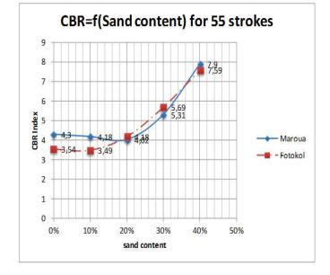
Figure 9. CBR Evolution according to sand content for 55 strokes (K1 and K2)
