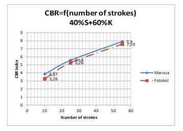
Figure 6. CBR Indexes according to the number of strokes for compound 40%S+60% (K1 and K2)
