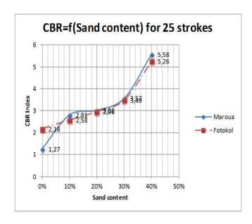
Figure 8. CBR index according to sand content for 25 strokes (K1 and K2)
