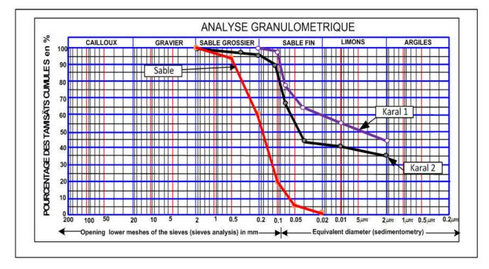
Figure 2. Results of the granulometric test
