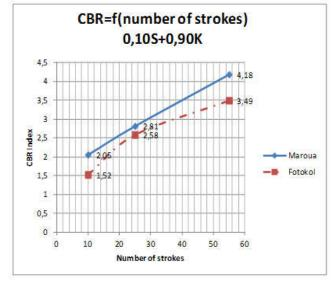
Figure 4. CBR Indexes according to the number of strokes for compounds 0%S+100% (K1 and K2), 10%S+90%(K1 and K2).
