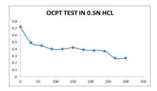
Fig. 5. OCPT Studies of Al 1100 in Different Concentration of HCl Solution
