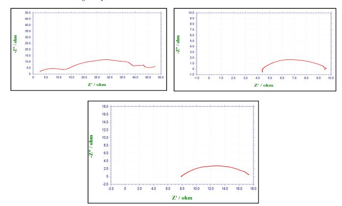
Fig. 8. Impedence studies of Al 1100 in different cocentration of NaCl solution
