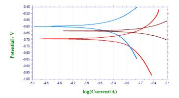
Fig. 4. Potentiodynamic Studies of Al 1100 in Different Concentration of NaCl Solution
