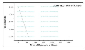
Fig. 6. OCPT Studies of Al 1100 in Different Concentration of NaCl Solution
