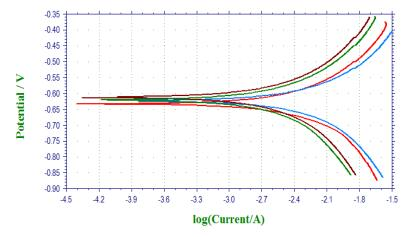
Fig. 3. Potentiodynamic Studies of Al 1100 in Different Concentration of HCl Solution
