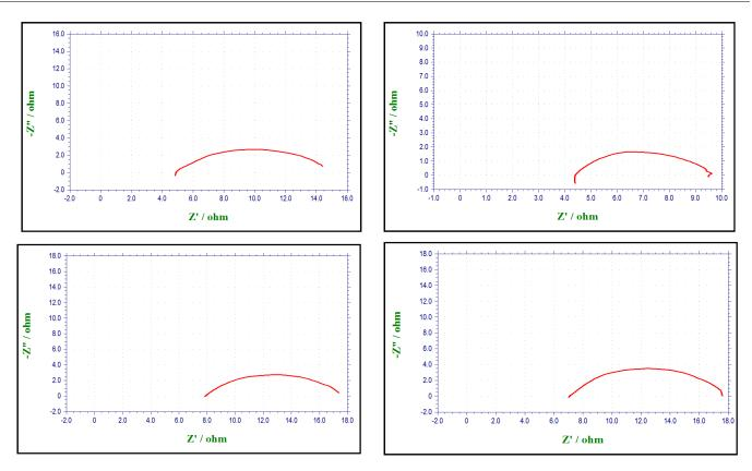
Fig. 7. Impedence studies of Al 1100 in different cocentration of HCl solution
