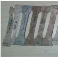
Figure 2. Variation of Tensile Strength with Fabricated Composites and Tensile Test Specimens
