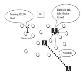
Figure 2. Routing attacks in WSN
