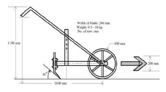
Figure a. Wheel hoe with sweep type blade
