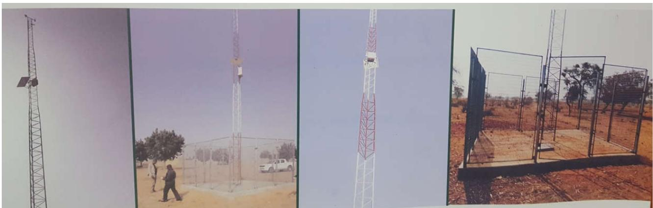
**Figure 4. Low Level Wind Shear Alert System (LLWAS) recently installed by NiMet at the**
