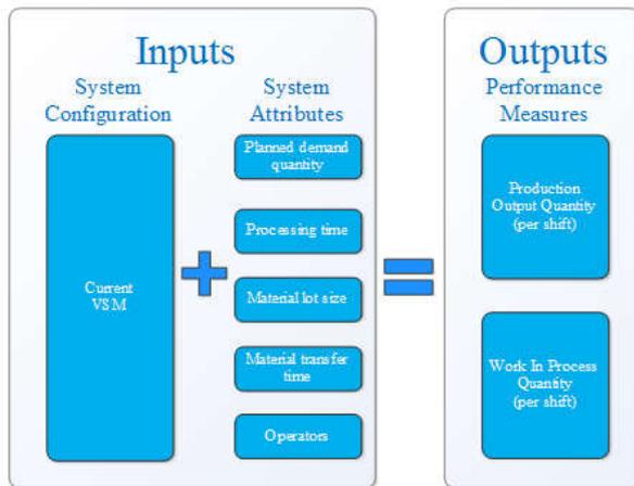
**Fig 2. Inputs and Outputs Variable of Current Production Simulation Model**
