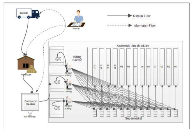
**Fig. 1. The flow of material and information among supplier, Warehouse, Compound/Kitting section and Assembly line section**
