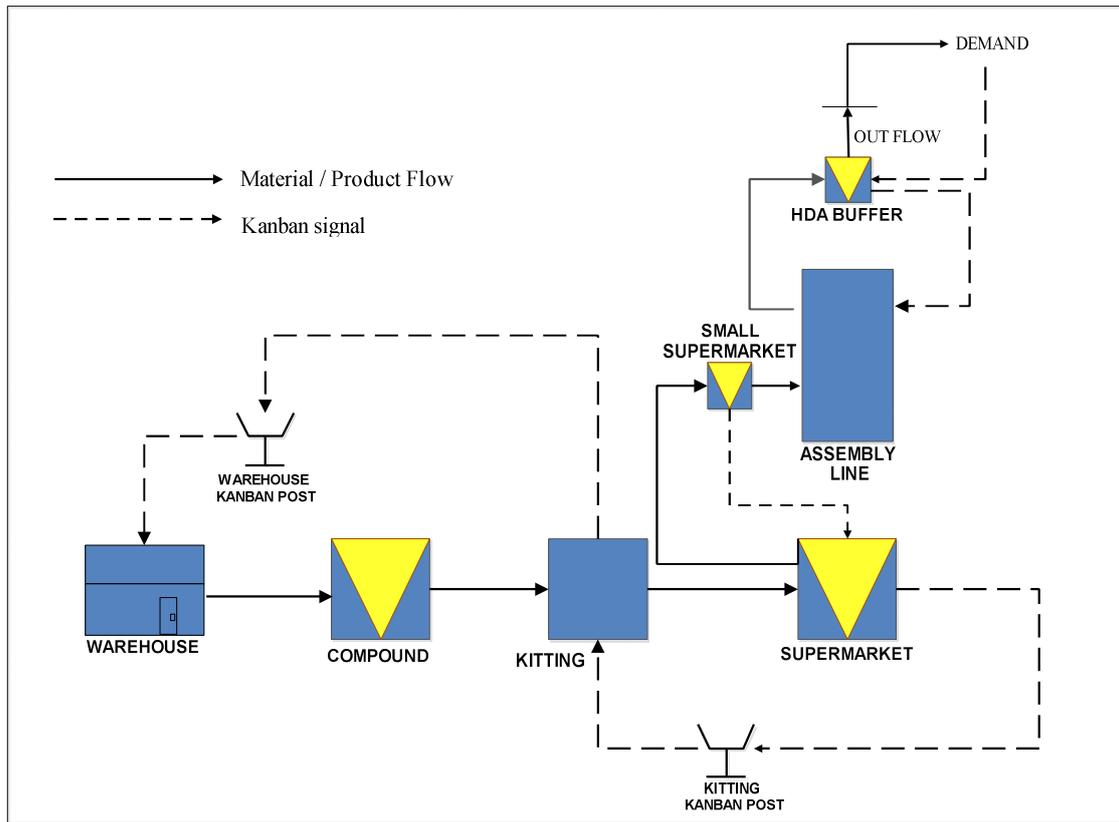
Fig 6. Material/Product flow for Simulation of Kanban System
