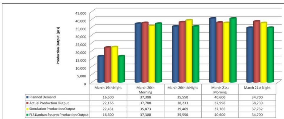
Figure 8. Comparison of Planned Demand and Production Output of Actual System, Simulation Model, and FLS Kanban System
