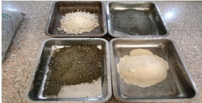
Figure 1. Raw materials used to manufacture laboratory cement
