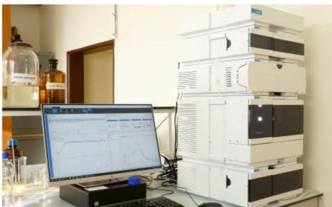
Figure 6. Agilent 1260 Infinity II chromatograph
