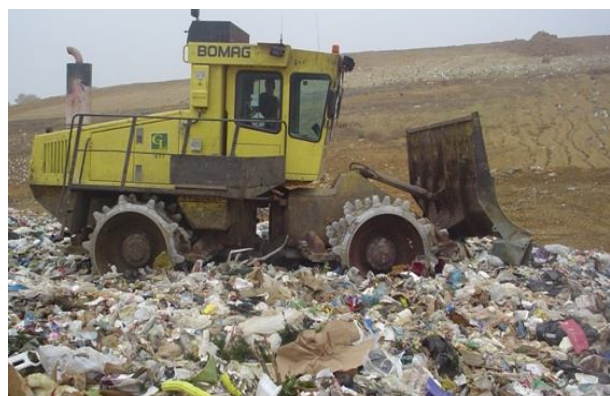
Fig. 6: Refuse compactor at a Solid Waste disposal site
