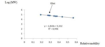
Figure 5. Determination of Molecular Weight of  $\alpha$ -glucosidase purified by electrophoresis
