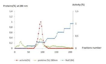
Figure 2. Anion exchange chromatography on Anx-Sepharose 4 fast flow gel of  $\alpha$ -glucosidase
