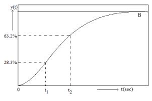
Fig.2. Typical process reaction curve
