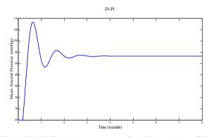
Fig.7. Z-N PI Closed loop response for infusion DP on CVS
