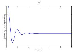
Fig.6. Z-N PI Closed loop response for infusion SNP on CVS
