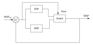
Fig.5.Swithing of Controller to regulate MAP
