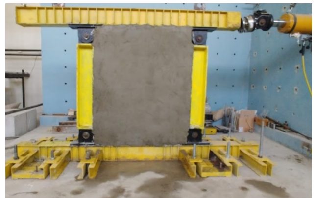
Figure 4. Masonry wall after plastering
